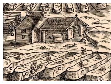
A typical nitrary (Germany, c.1580) with leaching deposits (() filled with decaying vegetable material mixed with manure. A worker collects efloresced saltpetre from deposits, transporting it then to be concentrated in the factory (B) boilers. (Source: https://en.wikipedia.org/wiki/Nitrary#/media/ File:Salnitrera.jpg)
